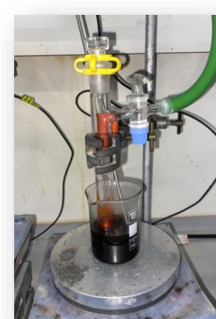
(Fig 13) Reaction set up for the formation of the phosphonium cation under nitrogen.
