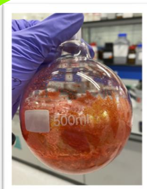
(Fig 9) The formed primary phosphine before extraction from round bottom flask.
